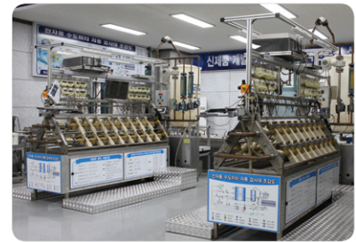
Electronic automatic water meter testbench 1,6 (Metrological Class horizontal R100 to R200) (15 to 50mm)
