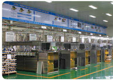
Electronic automatic water meter testbench 1,6 (Metrological Class horizontal R100 to R200) (15 to 50mm)
